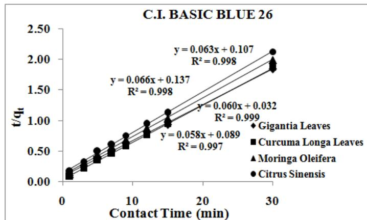
Figure 8: Pseudo-Second-Order Plot for C.I. Basic Blue 26 Adsorbed Onto Different Adsorbents
