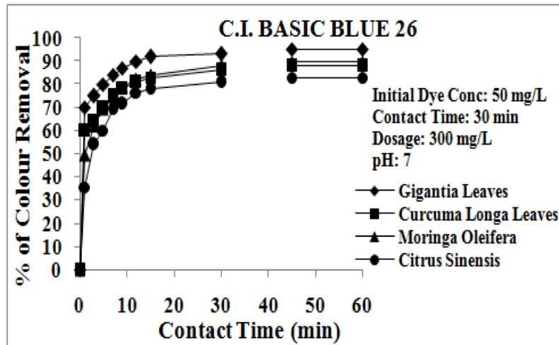
Figure 9: Interruption Kinetic Plot of C.I. Basic Blue 26
