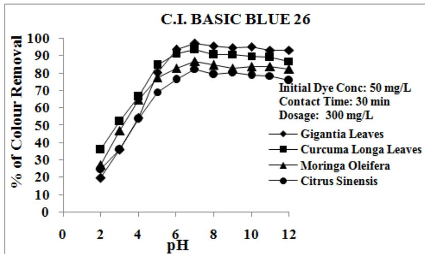
Figure 2: Response of C.I. Basic Blue 26 onto Adsorbents at Different Ph
