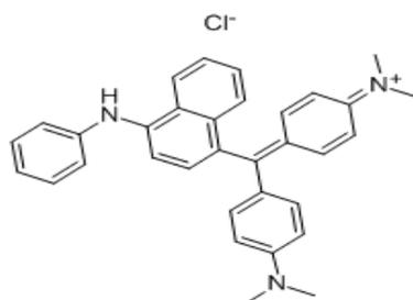
Figure 1: Chemical Structure of C.I. Basic Blue 26
