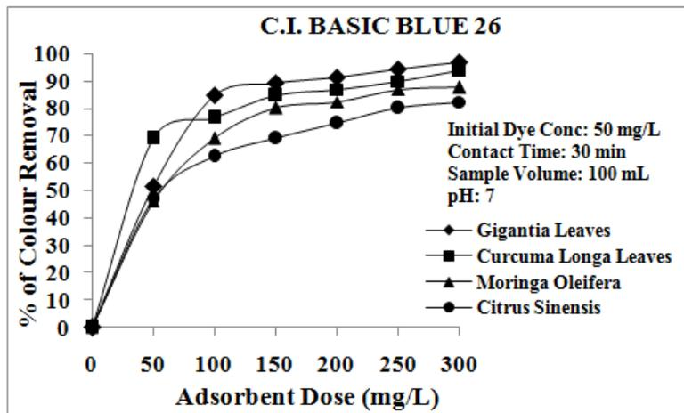
**Figure 3: Response of C.I. Basic Blue 26 to Adsorbents at Different Dosages (Ph=7)**
