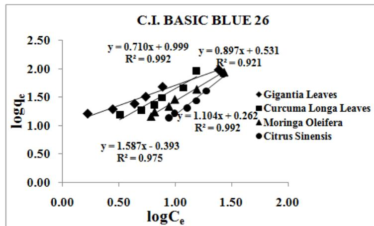
Figure 6: Linearised Plot of Sorption Isotherm of Freundlich Model for Various Adsorbents (C.I. Basic Blue 26)
