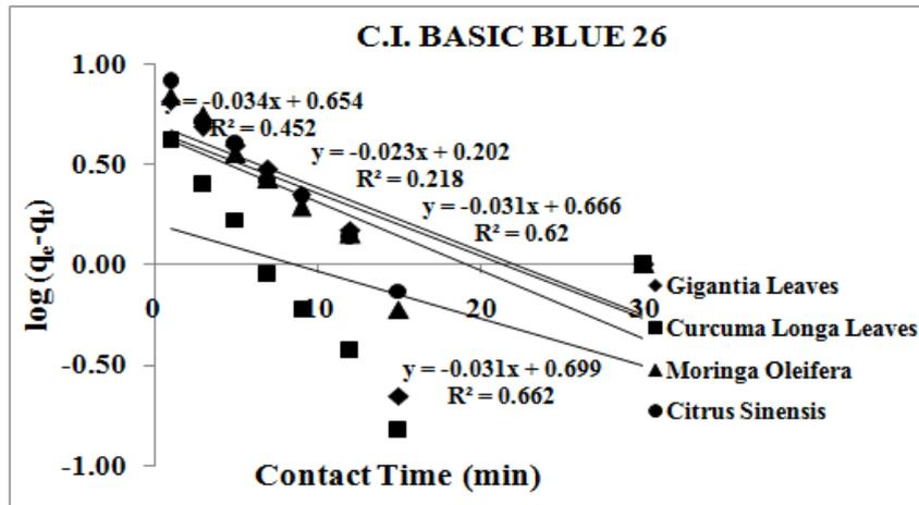
Figure 7: Pseudo-First-Order Plot for C.I. Basic Blue 26 Adsorbed Onto Different Adsorbents
