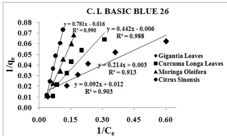
Figure 5: Linearised Plot of Sorption Isotherm of Langmuir Model for Various Adsorbents (C.I. Basic Blue 26)
