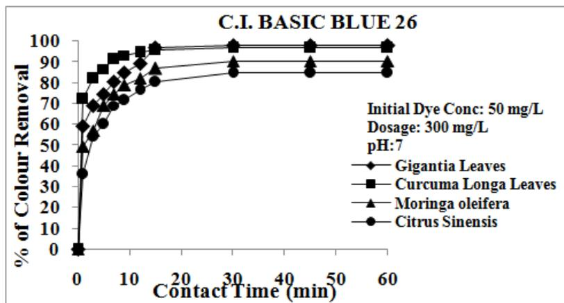
**Figure 4: Kinetics of Sorption of C.I. Basic Blue 26 onto Adsorbents at Different Contact Times (Ph=7)**
